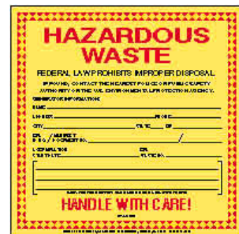
Figure 5.2: Hazardous Waste Shipping Label
